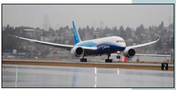
Boeing 787 landing at the end of its maiden flight, illustrating the flexibility of its wings.
