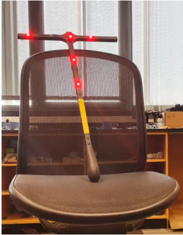
(a) Image of the motion detection calibration wand
