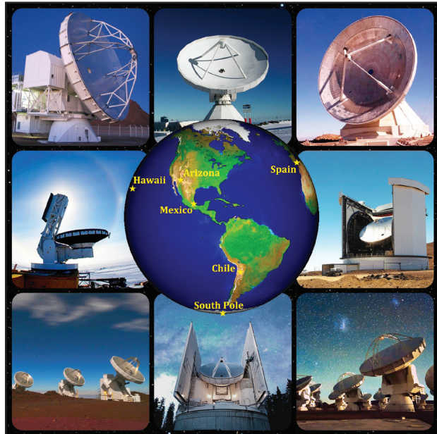
Figure 2. Synchronized telescopes across the globe form a virtual telescope called the Event Horizon Telescope that can achieve an unprecedented resolution. Figure courtesy of Kristy Johnson.
