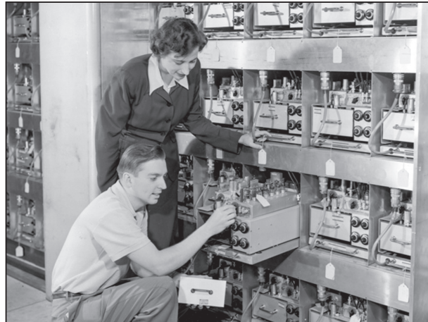
Margaret Butler and Rudolph Klein, an engineer at Oak Ridge National Lab, worked on the assembly of the ORACLE computer. Designed at Argonne and constructed at ORNL, ORACLE was in 1953 the world's fastest computer, multiplying 12-digit numbers in .0005 seconds.
