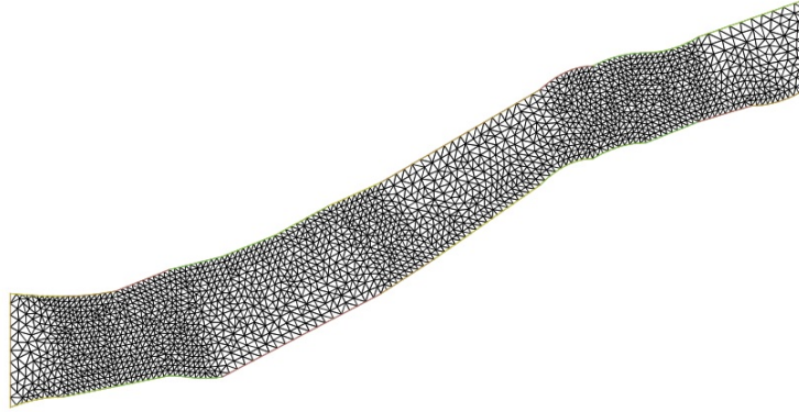
Figure 1: Shown above is a mesh of the domain (river).
