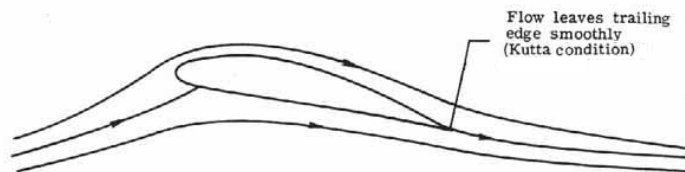
Figure 2: Inviscid flow over an airfoil with the Kutta condition applied. Note how the flow meets smoothly at the trailing edge. [15]
