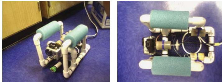
FIG. 2.1. Configuration of the Sea Perch used in this paper. Picture on the right is a top-down view, which shows the position of the three motors and how they are oriented.
