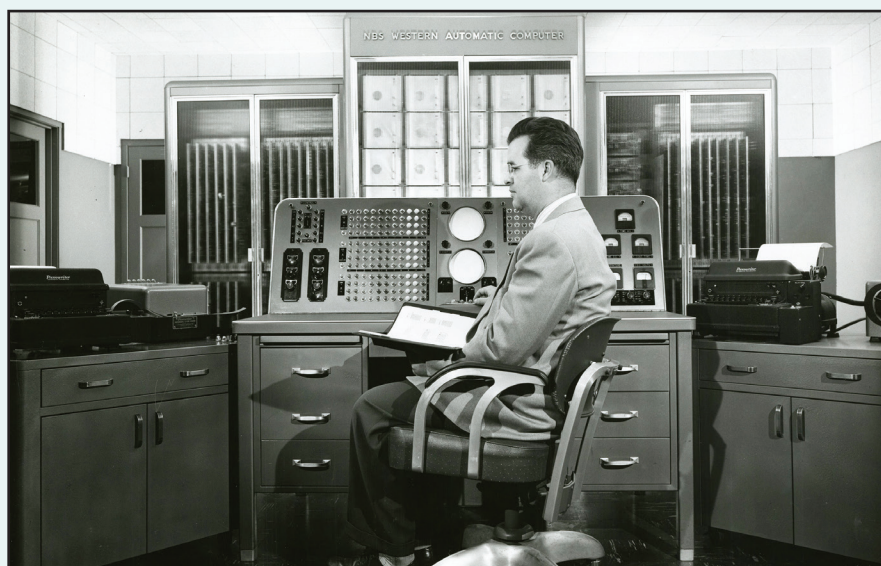
Figure 1. Harry Douglas Huskey works at the Standards Western Automatic Computer (SWAC), which he designed and constructed for the Institute for Numerical Analysis at the U.S. National Bureau of Standards. Figure courtesy of the National Institute of Standards and Technology Digital Archives, Gaithersburg, MD, 20899.
